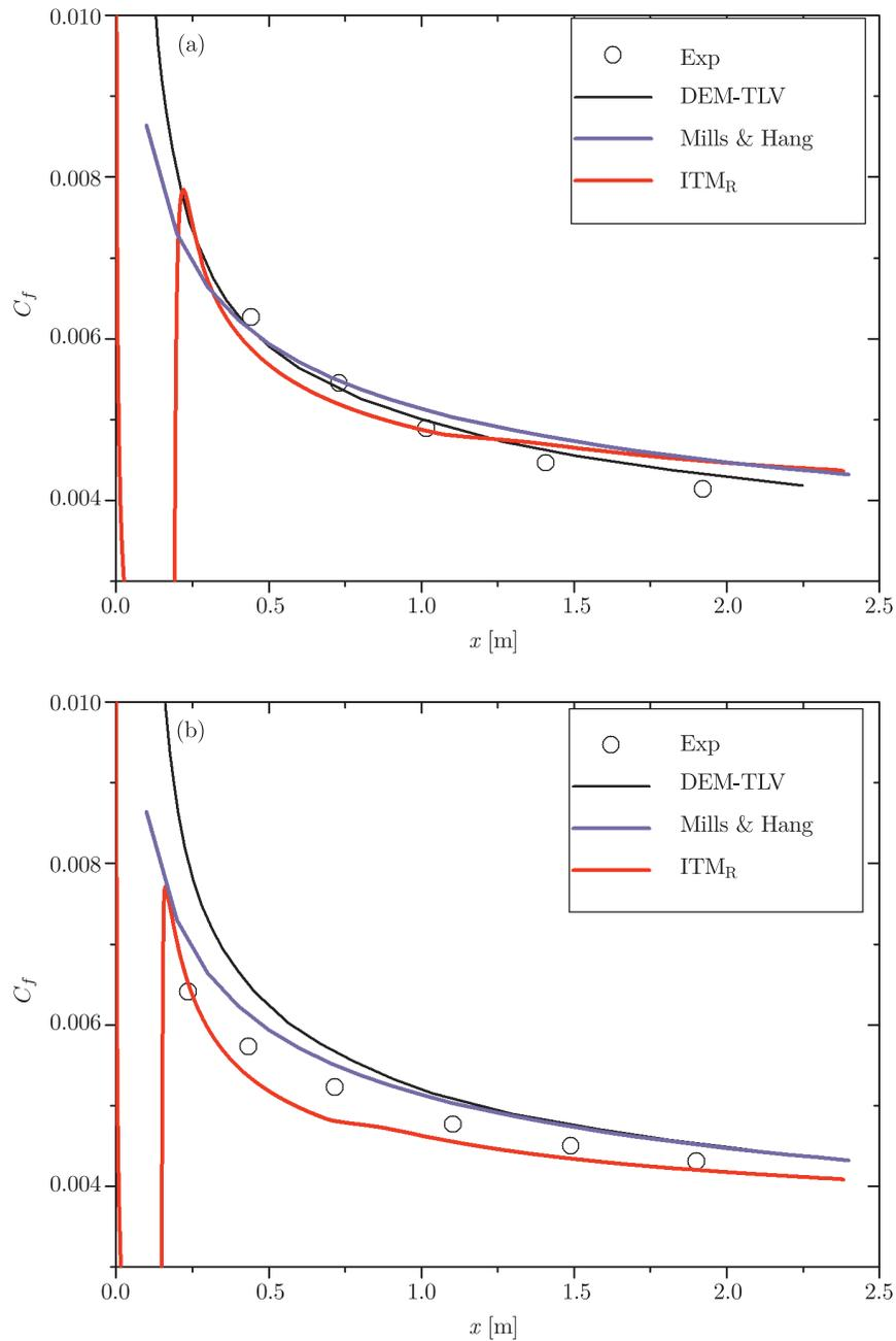
**Figure 1.** Skin friction coefficient distribution for zero-pressure gradient:
