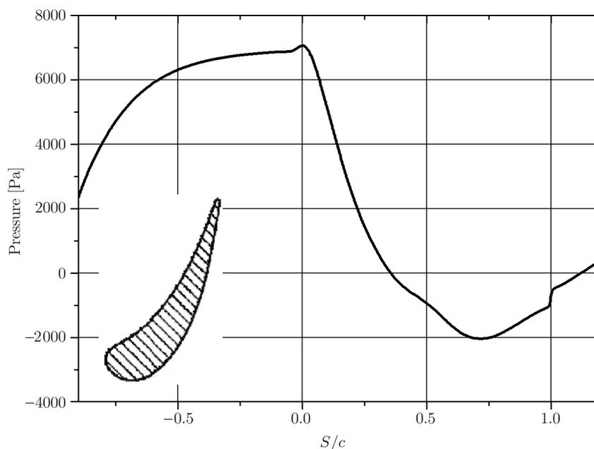
Figure 4. Pressure distribution for HPTV blade
