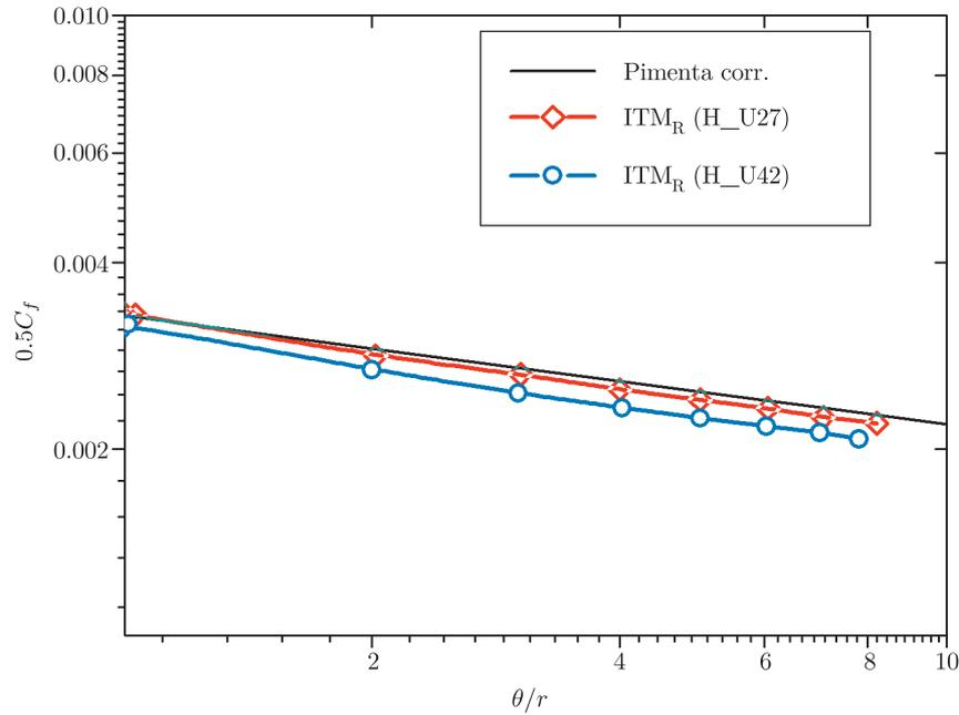
**Figure 2.** Skin friction coefficient distribution as function of  $\theta/r$  for zero-pressure gradient
