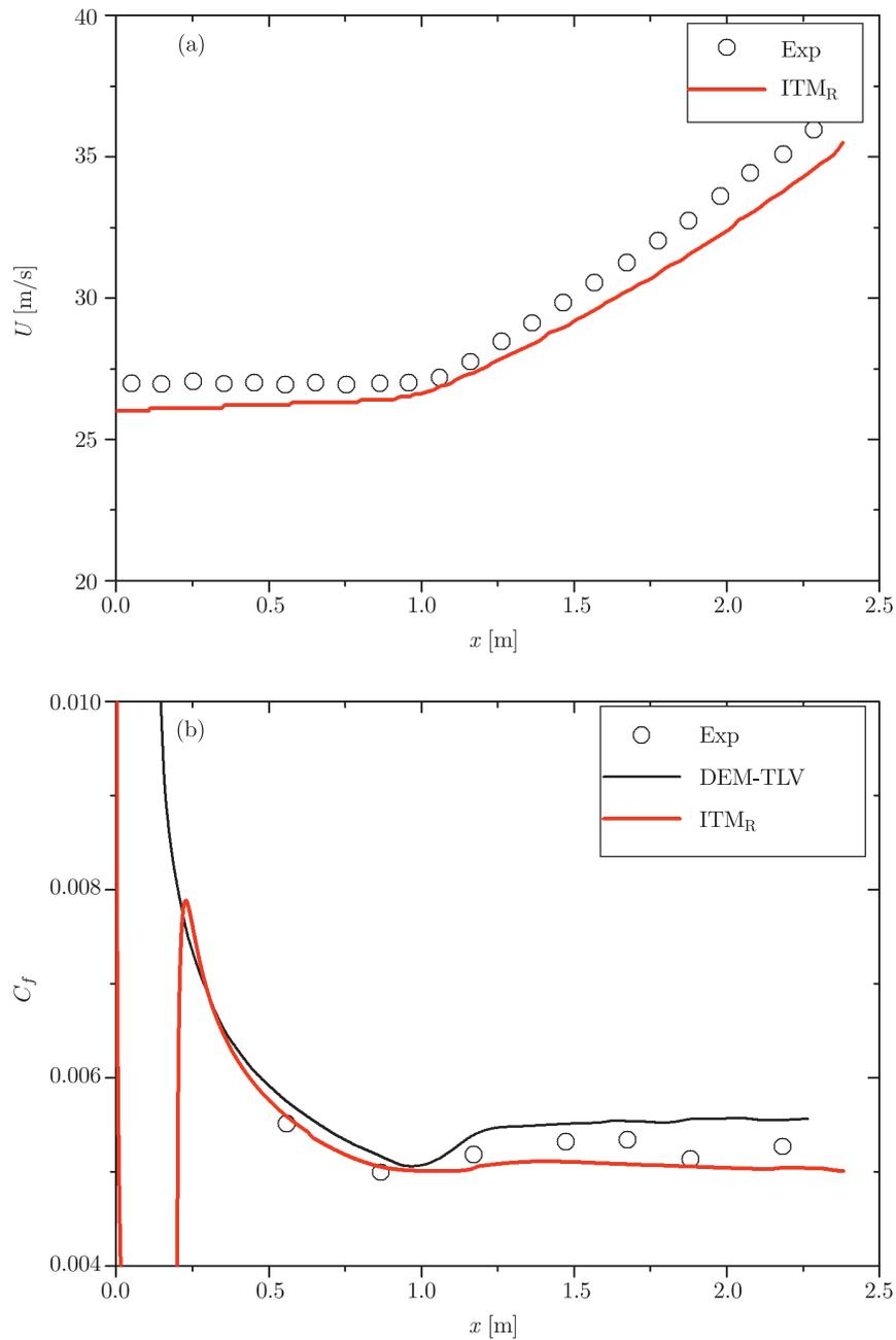
**Figure 3.** Freestream velocity distribution (a) and friction coefficient distributions (b) for non zero-pressure gradients flow
