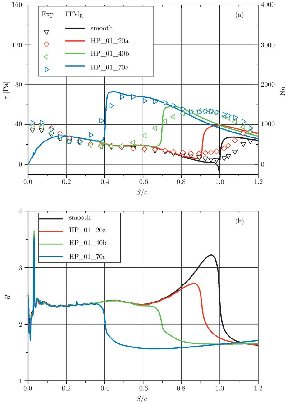
**Figure 5.** Skin friction (numerical results) and Nusselt number (experimental results) distributions (a), shape factor distributions (b) for various surface roughness for HPTV blade
