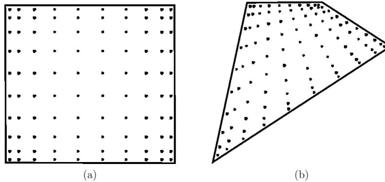
**Figure 4.** The arrangement of nodes of the Gauss-Legendre quadrature in (a) the basic square shape and (b) the modified shape
