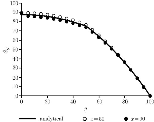
**Figure 8.** The distribution of stress in the square plate with variable density
