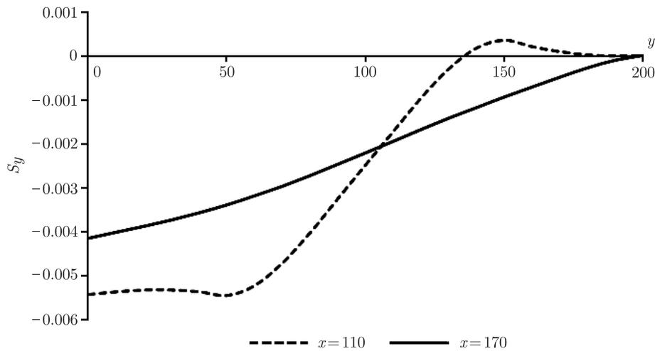
Figure 10. The stress distribution  $\sigma_y$  in two cross-sections of the domain
