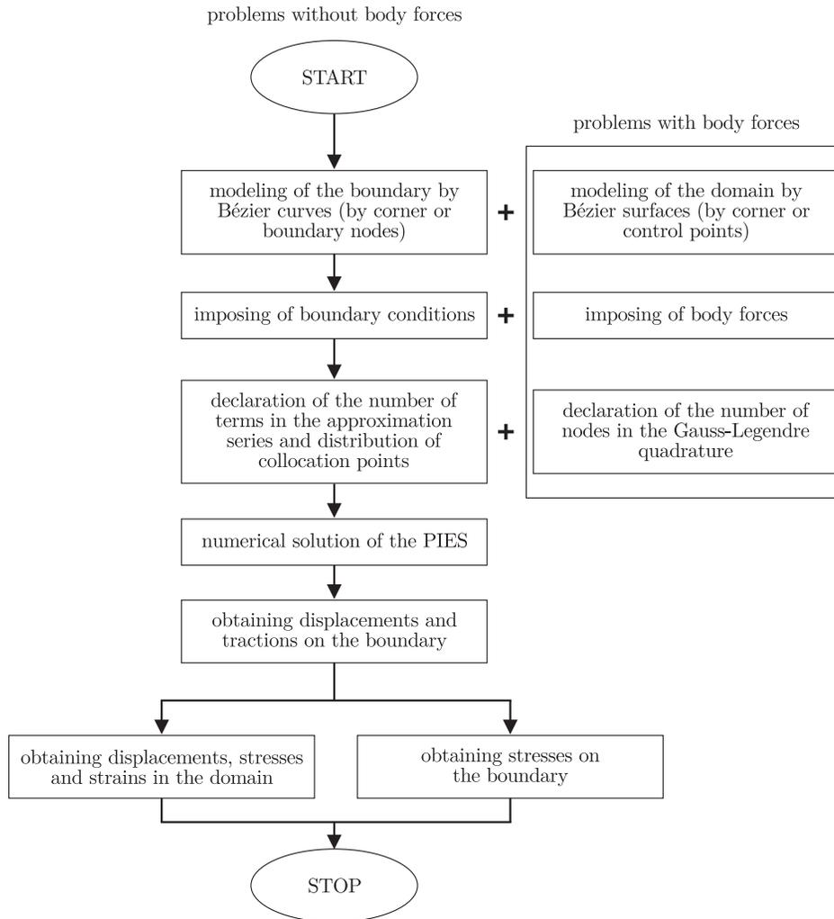
**Figure 1.** The process of the numerical solution of boundary problems of elasticity by the PIES
