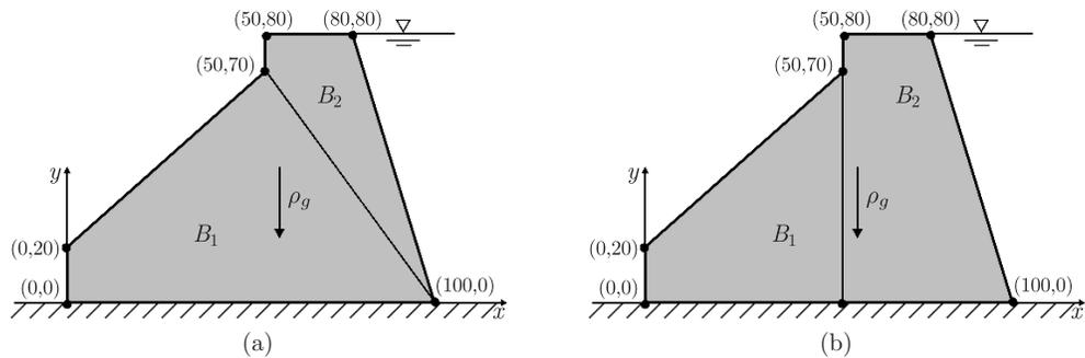
Figure 6. A dam modeled by two surfaces
