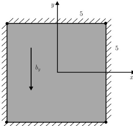
**Figure 5.** The plane body under gravitational force
