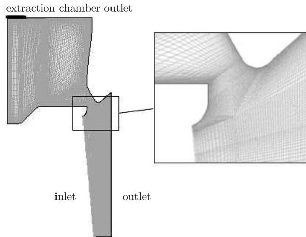
**Figure 2.** Geometry of interstage diffuser with extraction chamber, and calculation grid (variant without separation ring)
