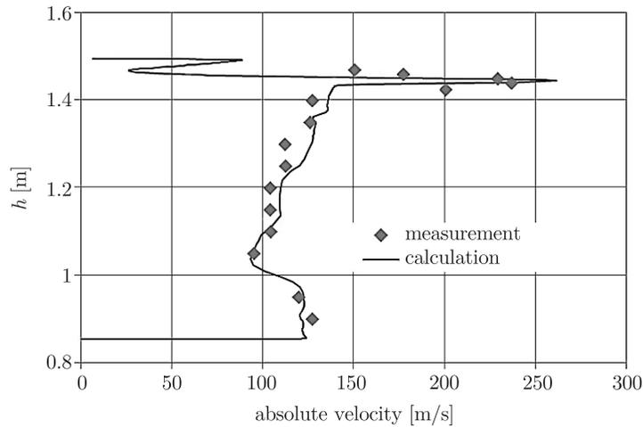
Figure 5. Comparing the calculated radial distributions of absolute velocity with those measured in a real turbine
