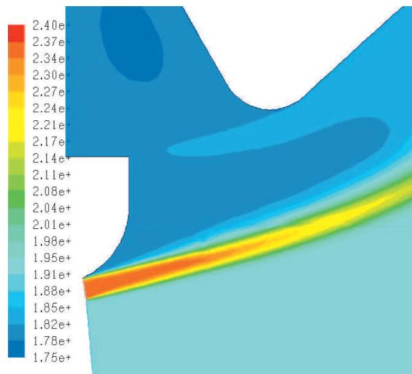
**Figure 7.** Total pressure distributions in steam extraction area: initial design
