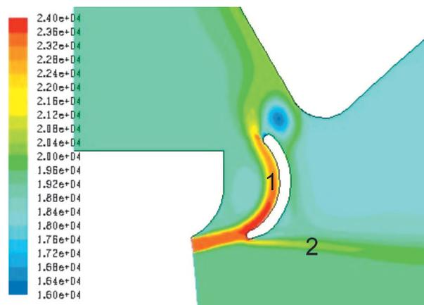
Figure 8. Total pressure distributions for ring mounted too high
