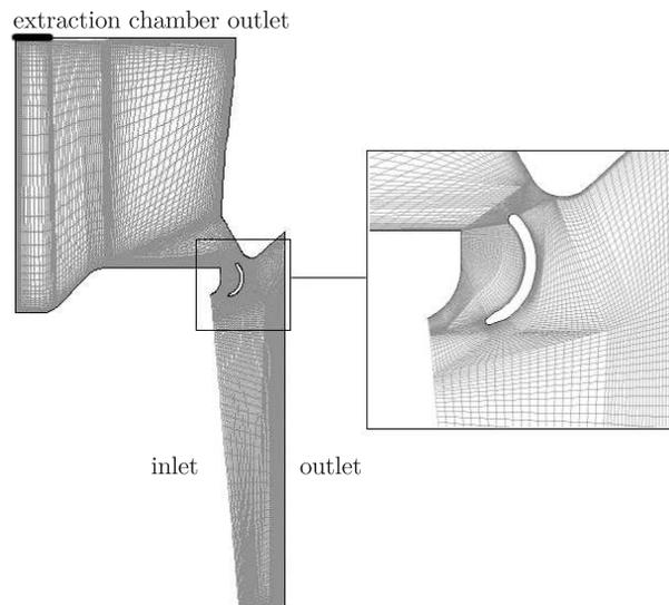
**Figure 3.** Geometry of interstage diffuser with extraction chamber, and calculation grid (variant with separation ring)
