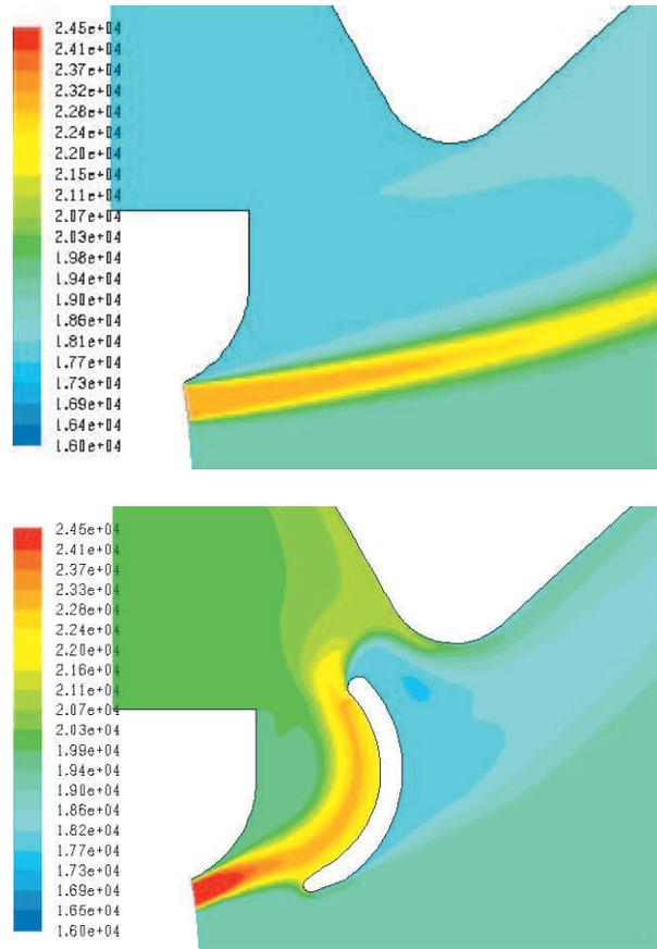
Figure 9. Comparing total pressure distributions before (top) and after modernisation (bottom)
