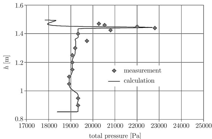
**Figure 4.** Comparing calculated radial distributions of total pressure with those measured in real turbine
