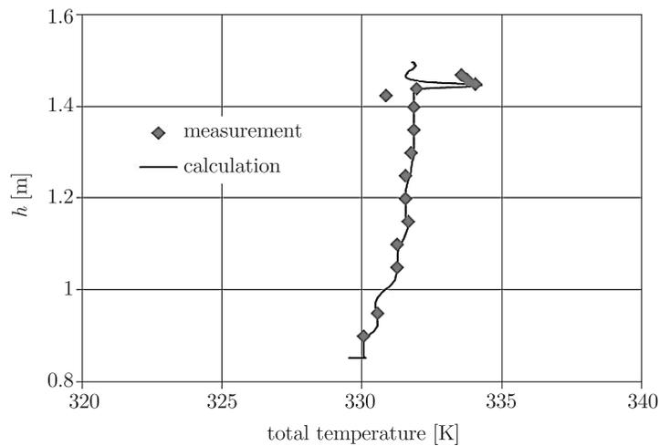
Figure 6. Comparing calculated radial distributions of total temperature with those measured in real turbine
