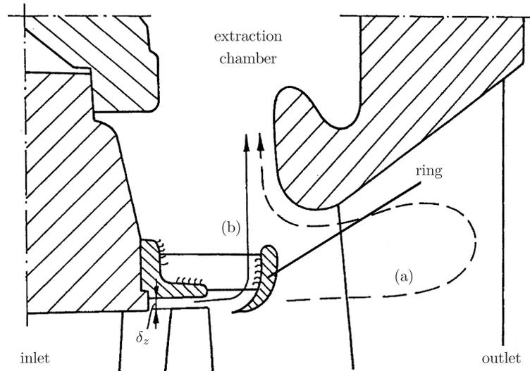
**Figure 1.** Turbine stage design in steam extraction area. The arrows indicate the leakage flow direction before (a) and after (b) modernisation
