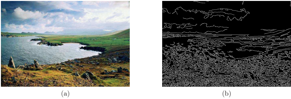
Figure 2. Representation of: (a) image, (b) its corresponding edge image produced by the Canny detector
